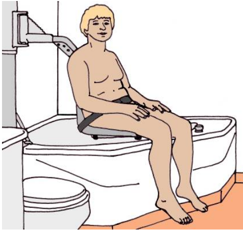
Hydraulic swiveling bath lift to transfer client in and out of the bathtub
